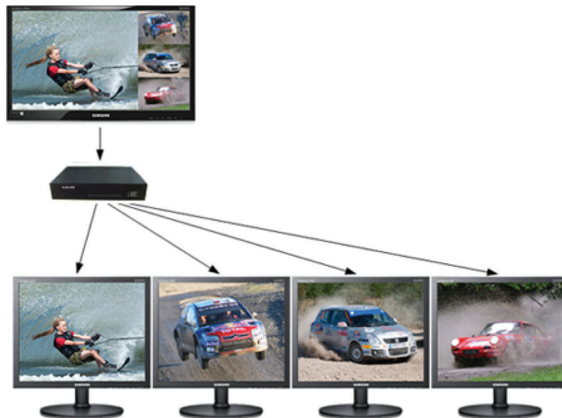
Figure 2-4. Crop input signal, upscale specific areas, and display on four separate screens.
